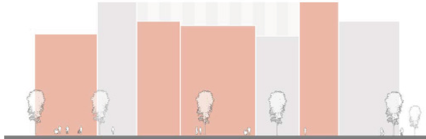
Figure 8.3: Elevation of easternmost block, showing the proposed distribution of red and grey brick across the facades (Source: AHMM).
