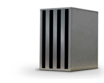
Our site safe carbon filters use panels of activated carbon to remove the malodourous gases within the commercial kitchen extract duct through the process of chemical adsorption. By installing adequate pre-filtration before our site safe filters, the carbon life span is greatly increased, allowing it to nullify malodours at optimum efficiency for much longer.
