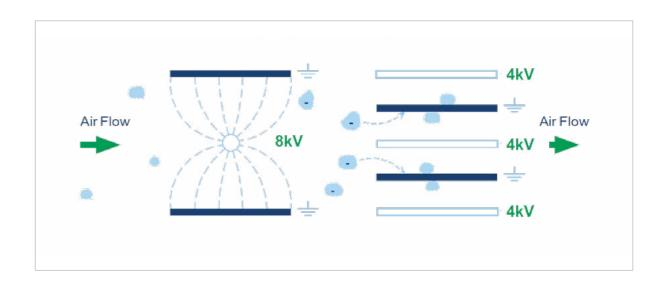
The above diagram shows, in a basic visual, how an electrostatic precipitator works. As air passes into the combined ioniser / collector cell, the particulates in the air stream are polarised. As they continue through the ioniser and
