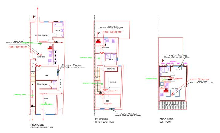
compliant fire doors between the kitchen and the stairs will be installed. Smoke and carbon monoxide alarm detectors will be installed that would follow the current regulations. Emergency lighting will be installed throughout the building. Secondary emergency exit windows will be available on each floor.
