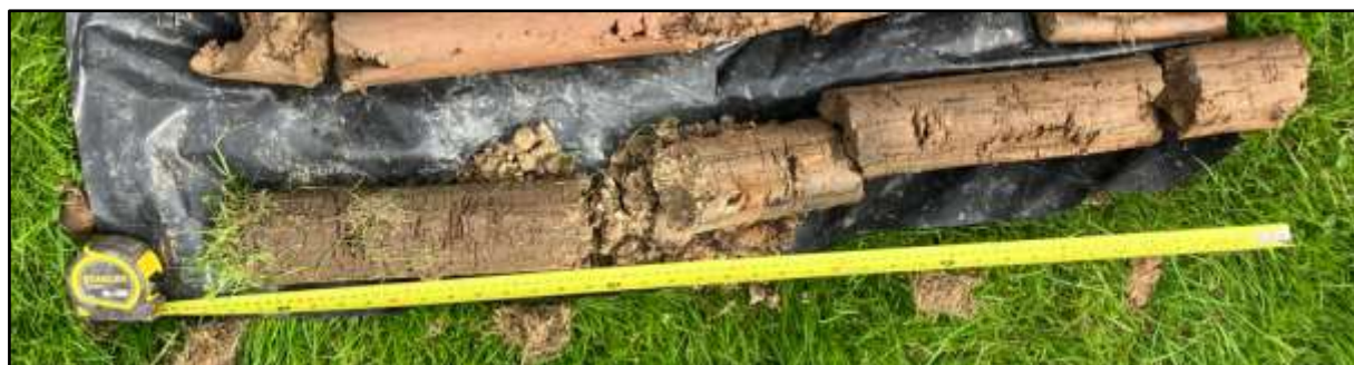
Figure 5-A: Arisings of topsoil and Made Ground 0.0-1.0m depth from WS05
