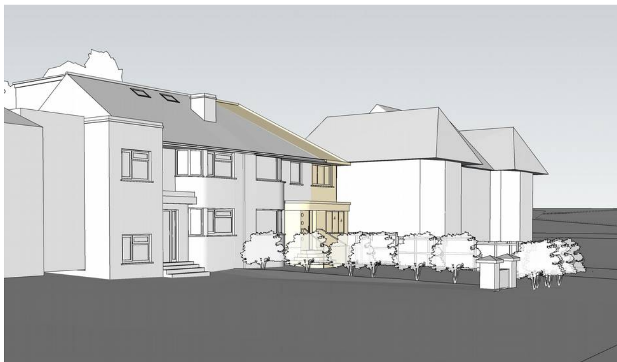
Proposed oblique view looking south east showing curved front projection in relation to existing curved bay windows of house
