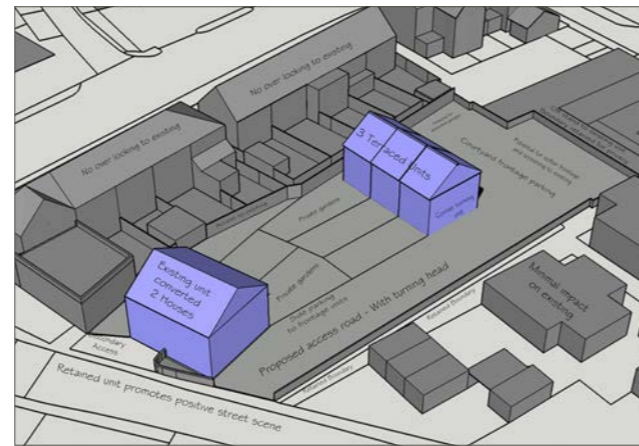
Exploring the feasibility of returning frontage units at 1-3 Chequer Lane to a pair of semi detached cottages with a terraced 3 block to the rear
