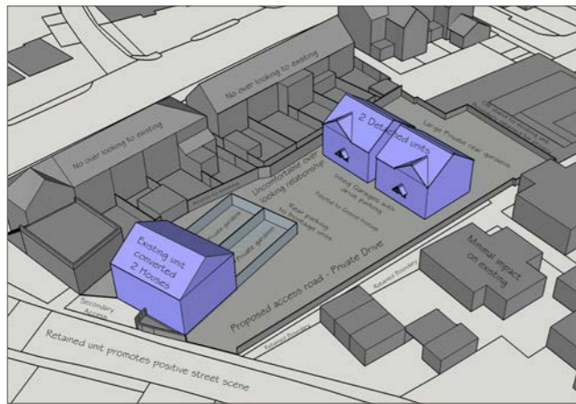
Initial 3D modelling exploring the feasibility of returning frontage units to a pair of semi detached cottages with detached larger scale / footprint dormer bungalows or similar to the rear. Access to No 217 Ormskirk Road's garage compromised
