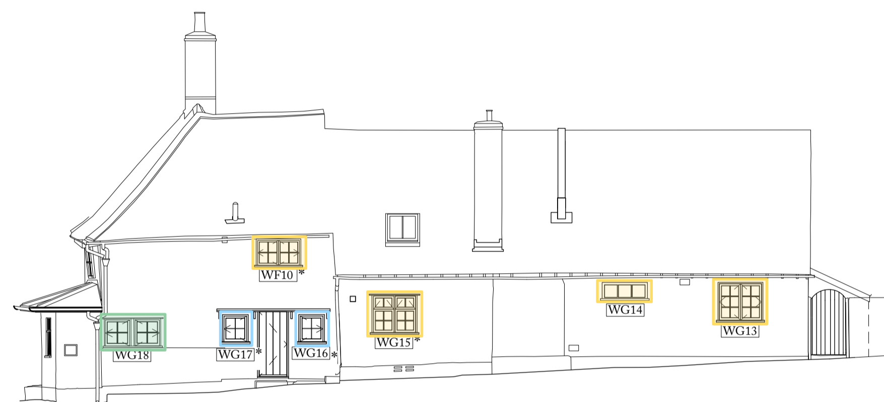
+30.00 Datum 4 EAST ELEVATION As Proposed, 1:100 * = Frosted Glazing
