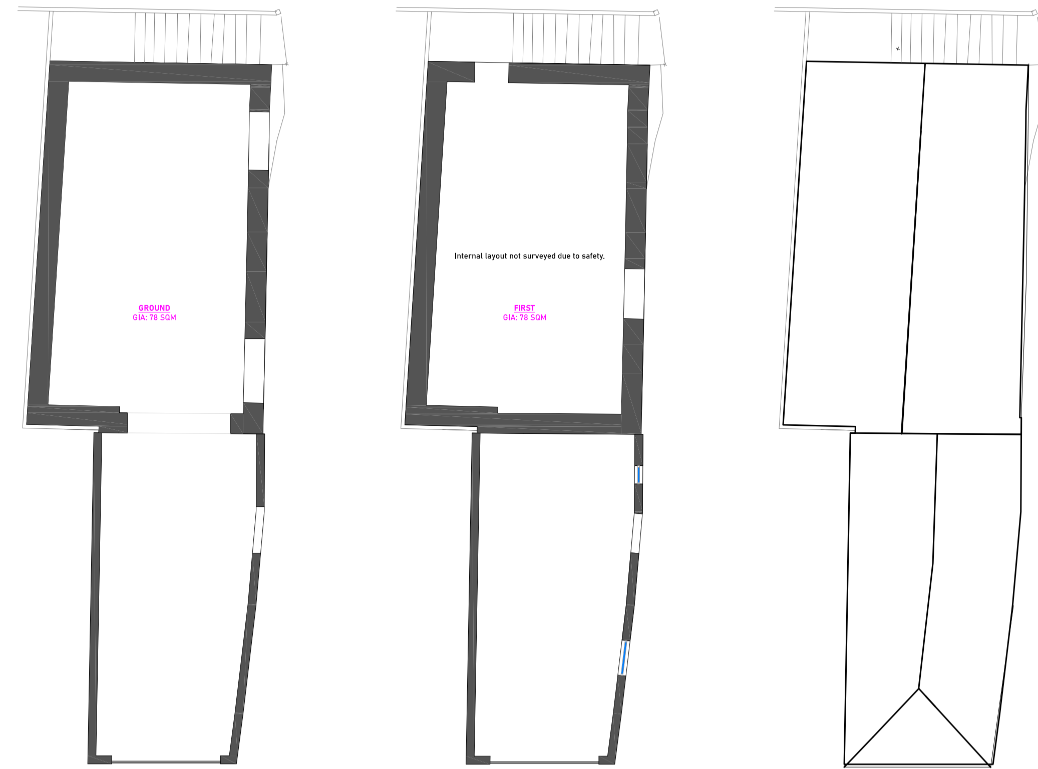
EXISTING Ground Floor Plan Scale: 1:100 EXISTING First Floor Plan Scale: 1:100 EXISTING Roof Block Plan Scale: 1:100
