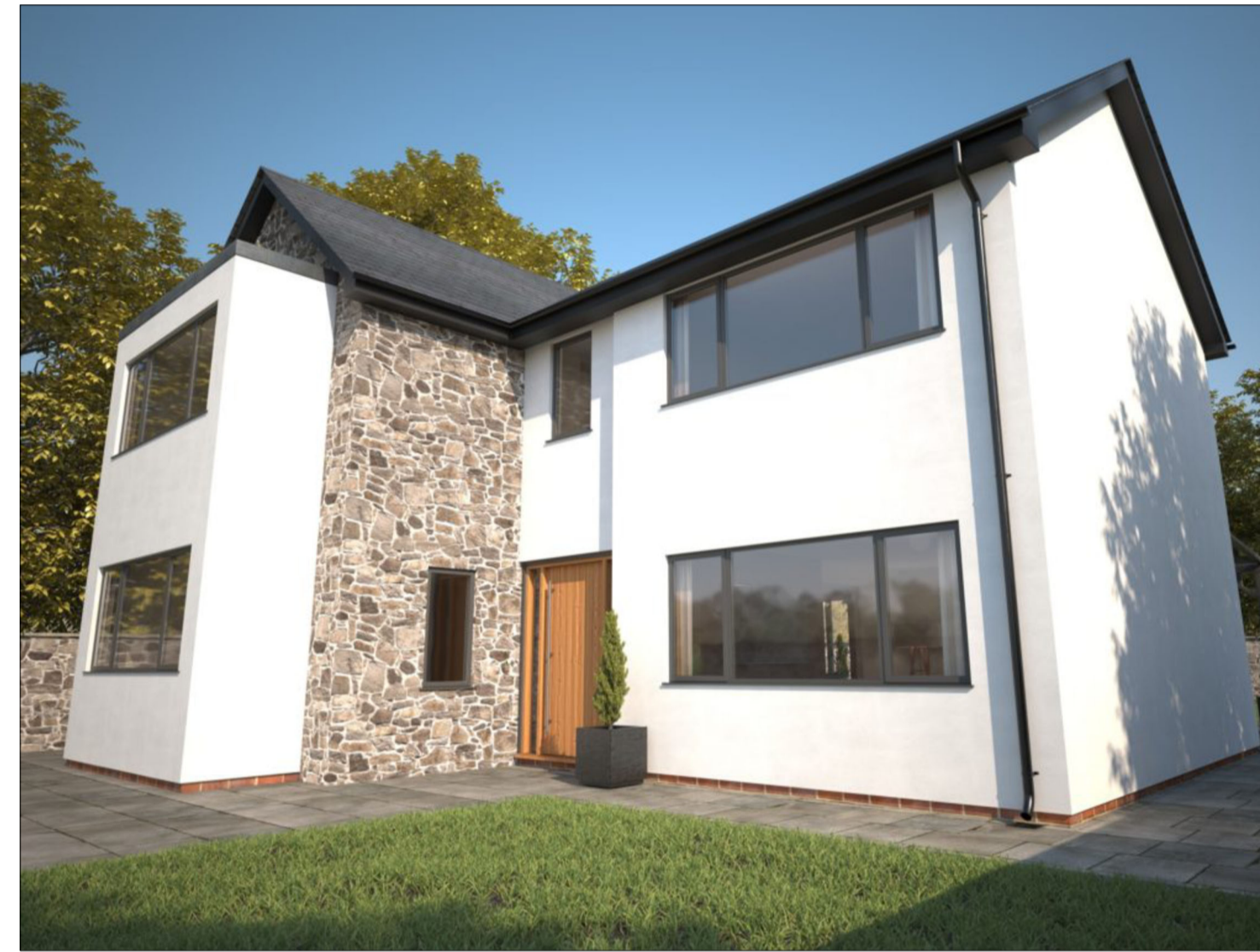
IMAGE 02 - Reference Project Showing Rubble Stone Facade, Slim Anthracite Windows, Slate Roof & White Render.
