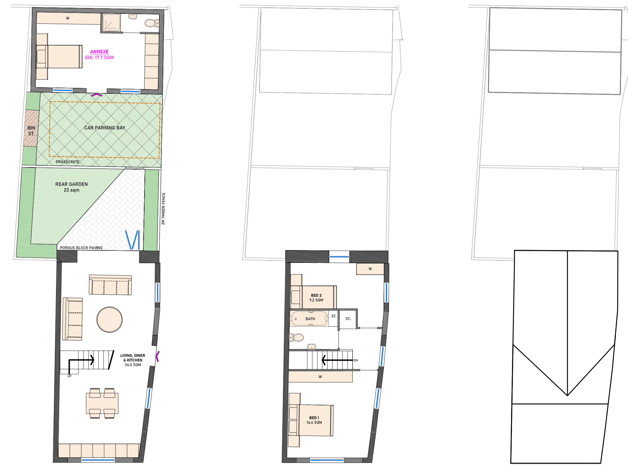
PROPOSED Ground Floor Plan Scale: 1:100 PROPOSED First Floor Plan Scale: 1:100 PROPOSED Roof Block Plan Scale: 1:100
