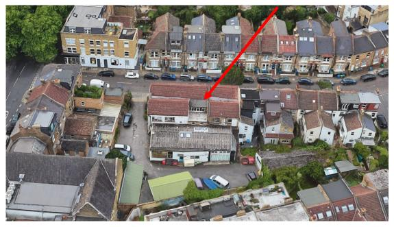
The proposal is to change the small amount of existing flat roof at second floor level to a pitched roof, to match the adjoining pitch on either side. The remaining element of flat roof at first floor would remain, but a glass balustrade would be added at the edge of this part of
