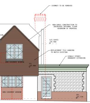
FLANK (SOUTH) ELEVATION As Proposed
