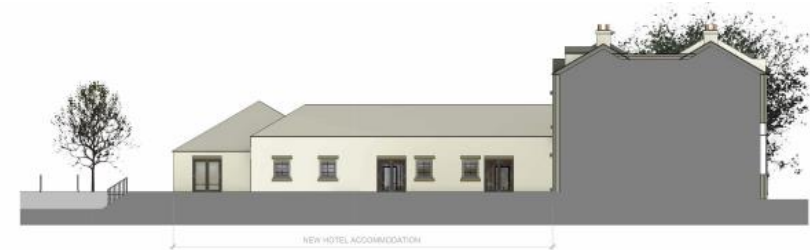
Proposed East Elevation with new doors to suites
