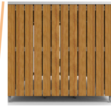
Proposed 2.0m high timber fence and gates to bin store Fence and gates to match cycle store
