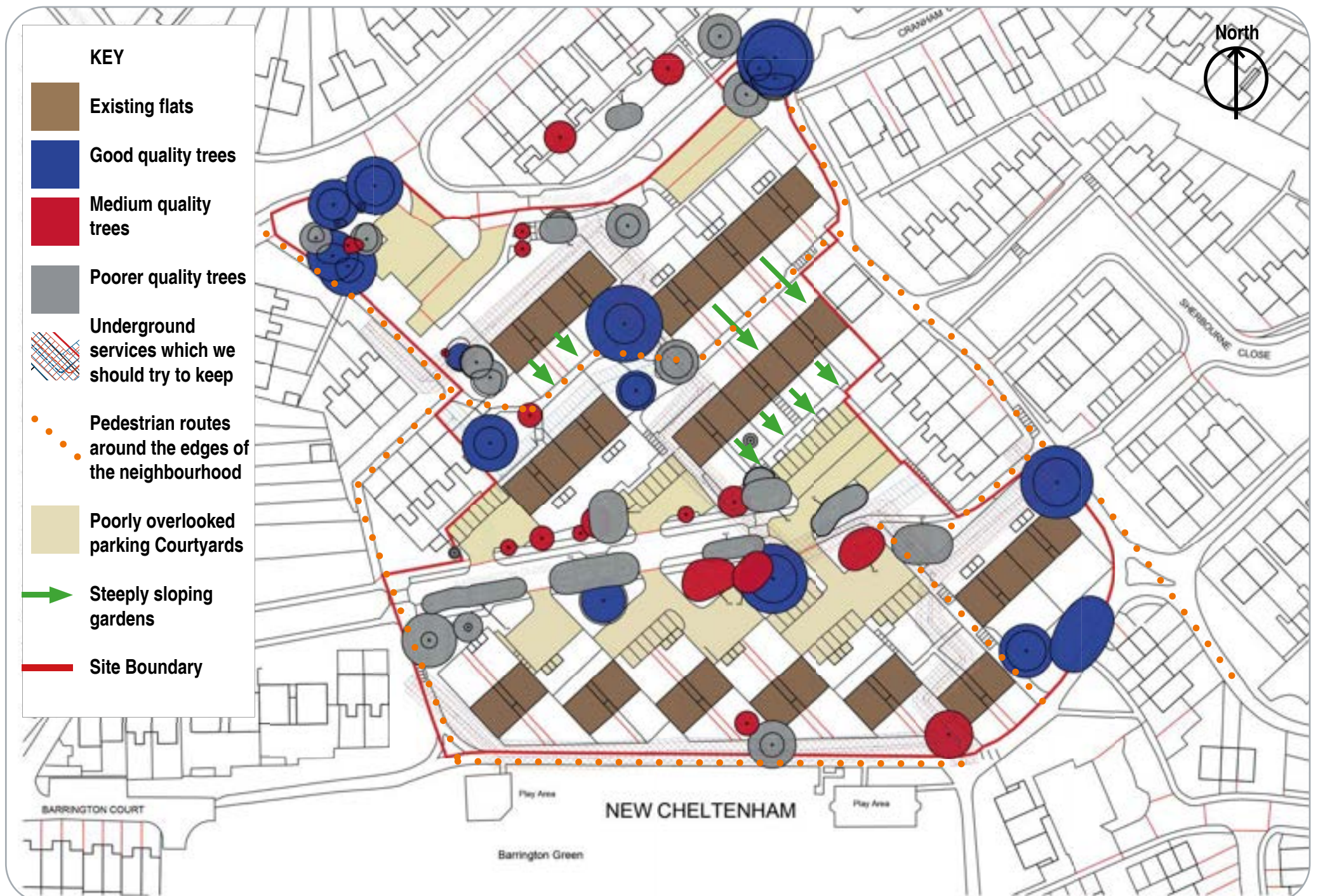
Diagram showing potential constraints and opportunities to the regeneration of the area
