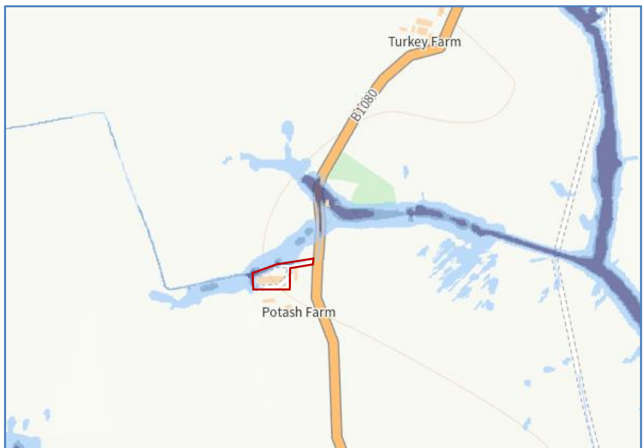
Figure 3.2 – Surface Water Indicative Flood Mapping
