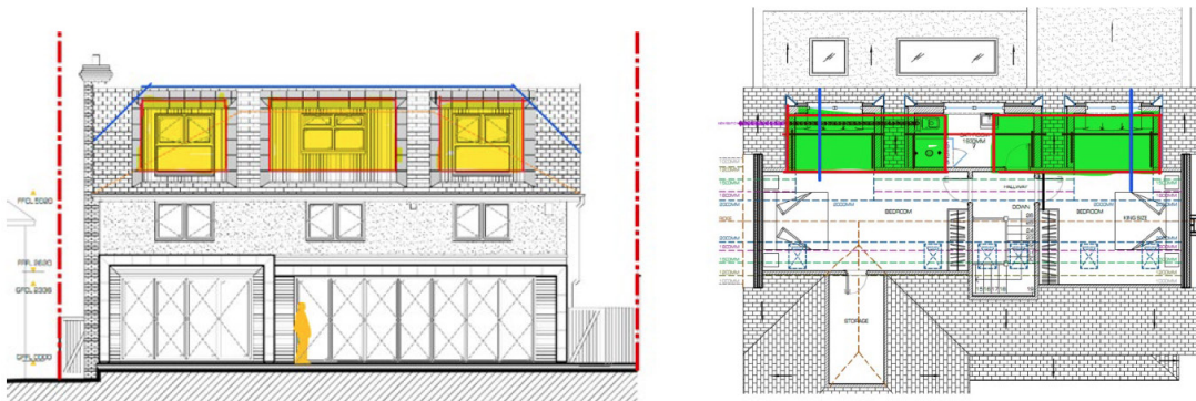
Figure 2 - Loft Plan and Rear Elevations with reduced dormers outlined
