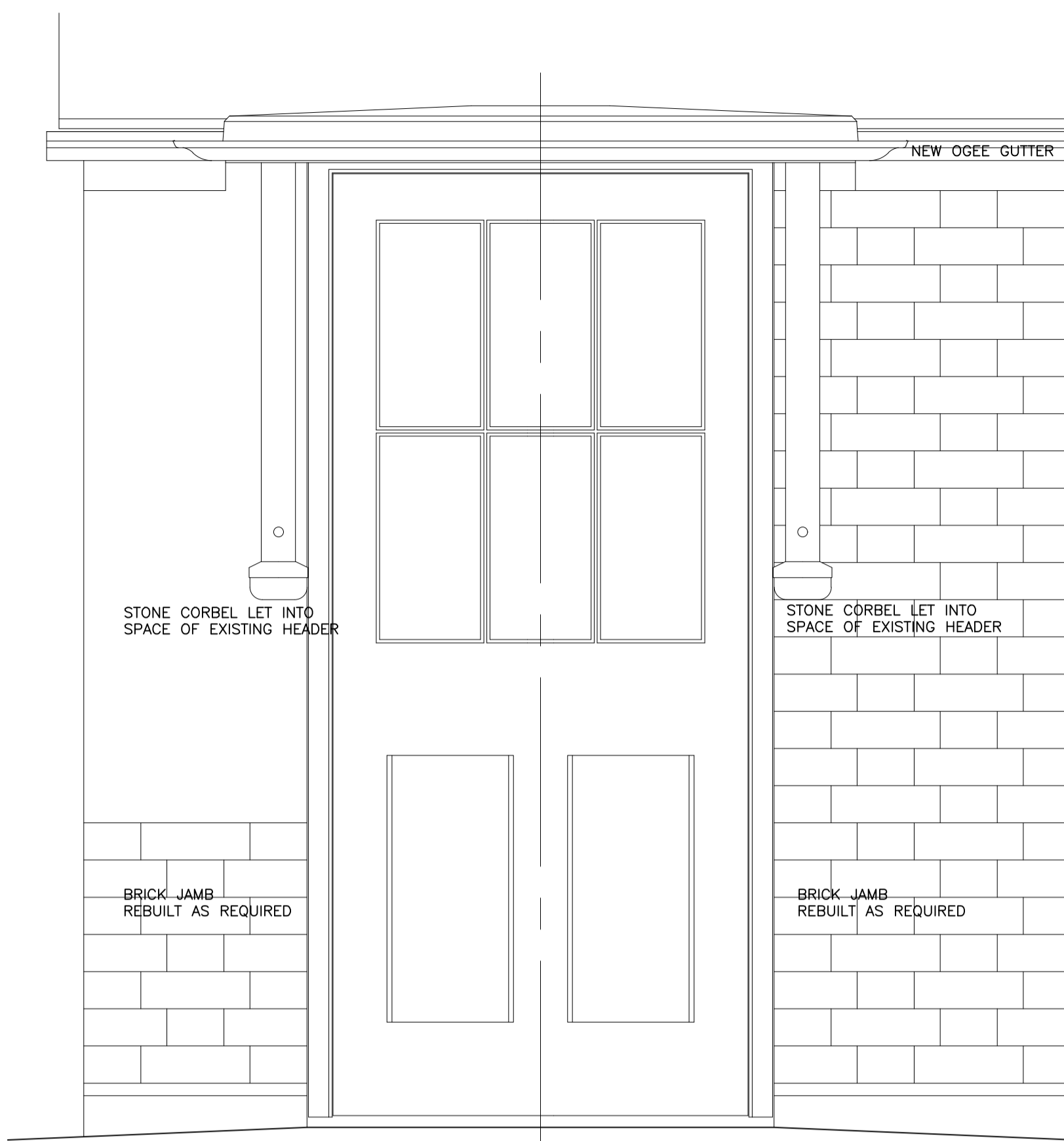
1:10 SCALE ELEVATION OF EDG/03
