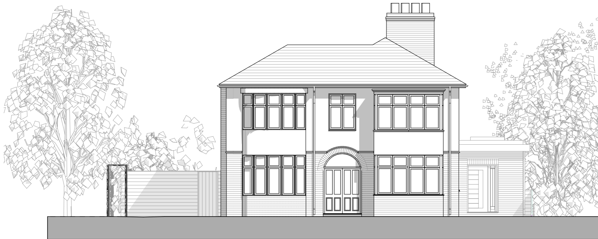
Proposed South Front Elevation 1:100
