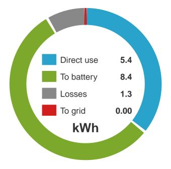
This graph shows the modelled profile of electricity generated by the PV array on a selected day (March 27th). On this day the PV system is expected to generate 15.1 kWh. Of this, 5.4 kWh (36%) is used directly in the property, 9.7 kWh (64%) is stored in the battery for later re-use, and 0 kWh (0%) is exported to the grid.
