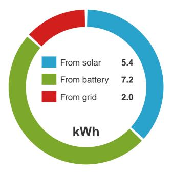
This graph shows modelled consumption data over the course of the selected day (March 27th). Total electricity consumption on this day was 14.6 kWh, of which 5.4 kWh (37%) is expected to be supplied directly by the solar array, and a further 7.2 kWh (49%) drawn from the battery storage system. The remaining 2 kWh (14%) is imported from the grid.
