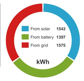
The property is expected to consume 4500kWh of electricity each year. Around 34% of this (1542 kWh) is expected to be supplied directly by the solar array. Another 31% (1397 kWh) is supplied from the storage battery. The remaining 35% (1575 kWh) is supplied from the grid.
