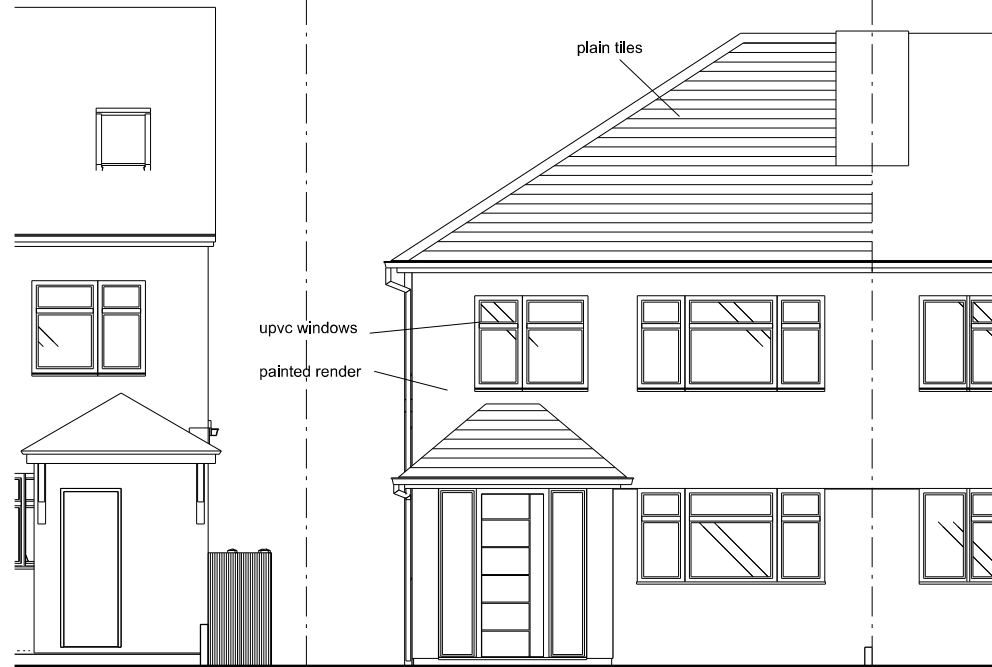
Existing Front Elevation
