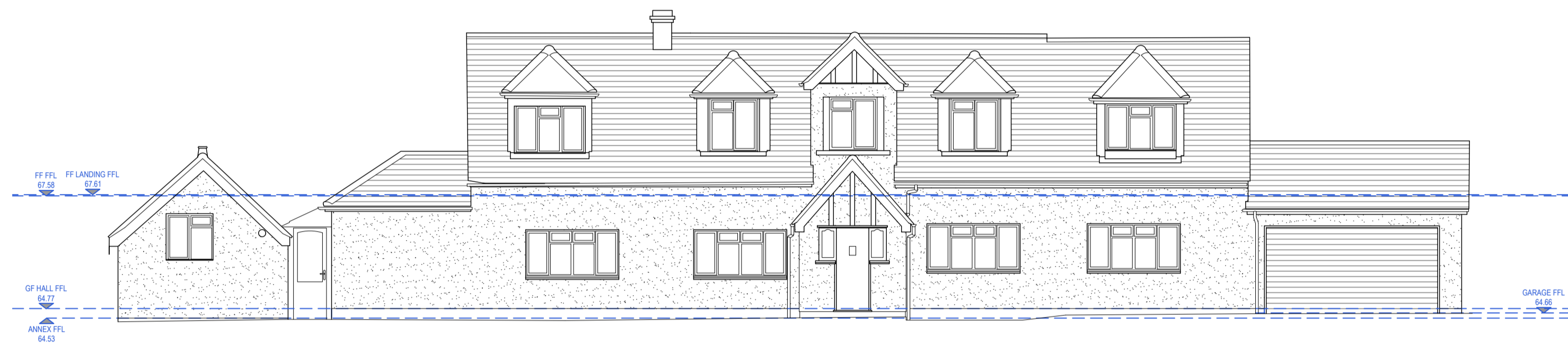
Existing Front Elevation - 1:100 @ A1
