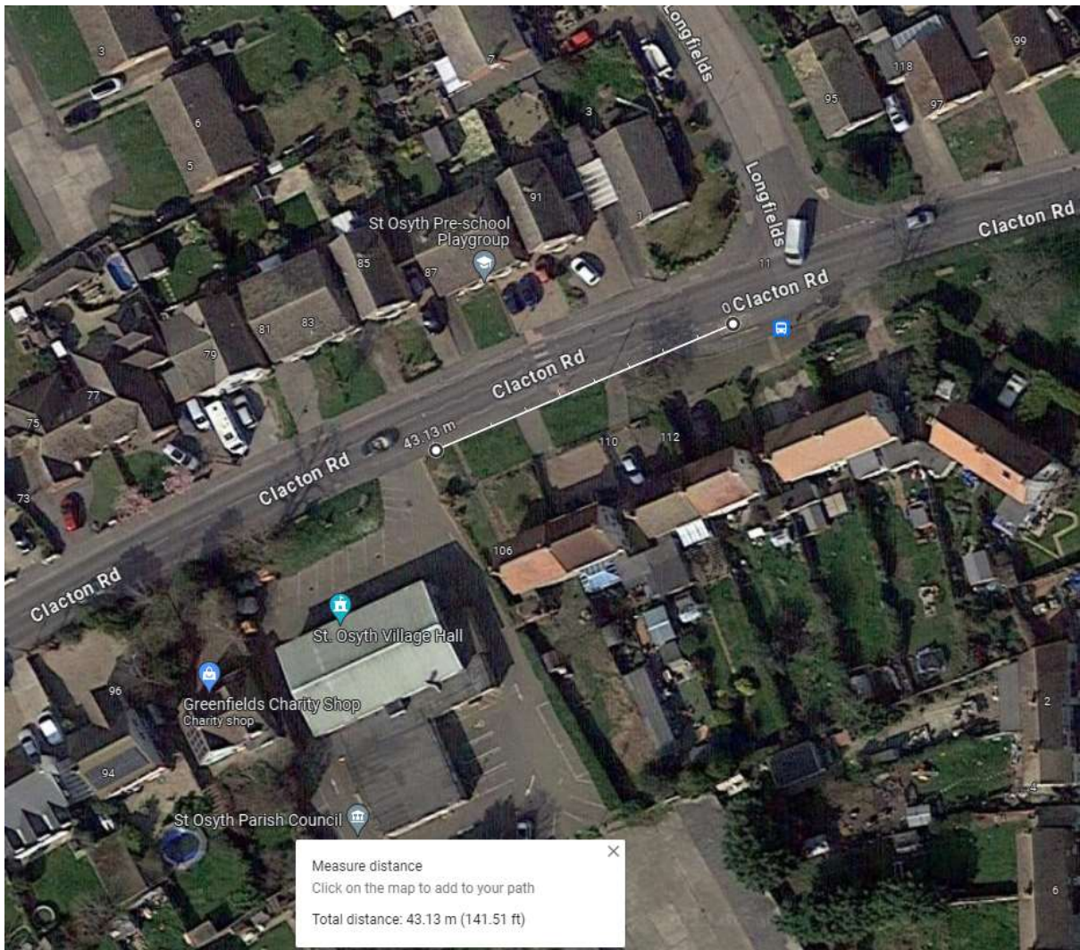
Fig. 2 – 30mph, 43m visibility splay distance looking north east
