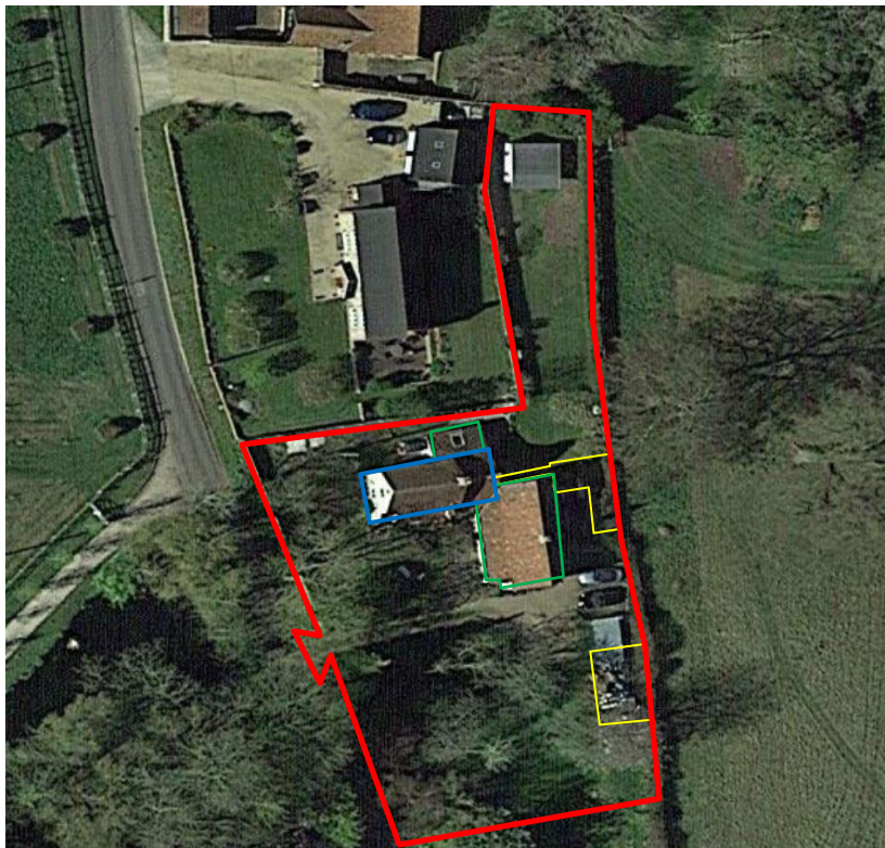
Figure 1 : Aerial photo of site plan (not to scale) showing site (outlined red), historic building (blue) and more modern additions (green) and location of proposed works (outlined yellow), from North to South (North is up the page):
