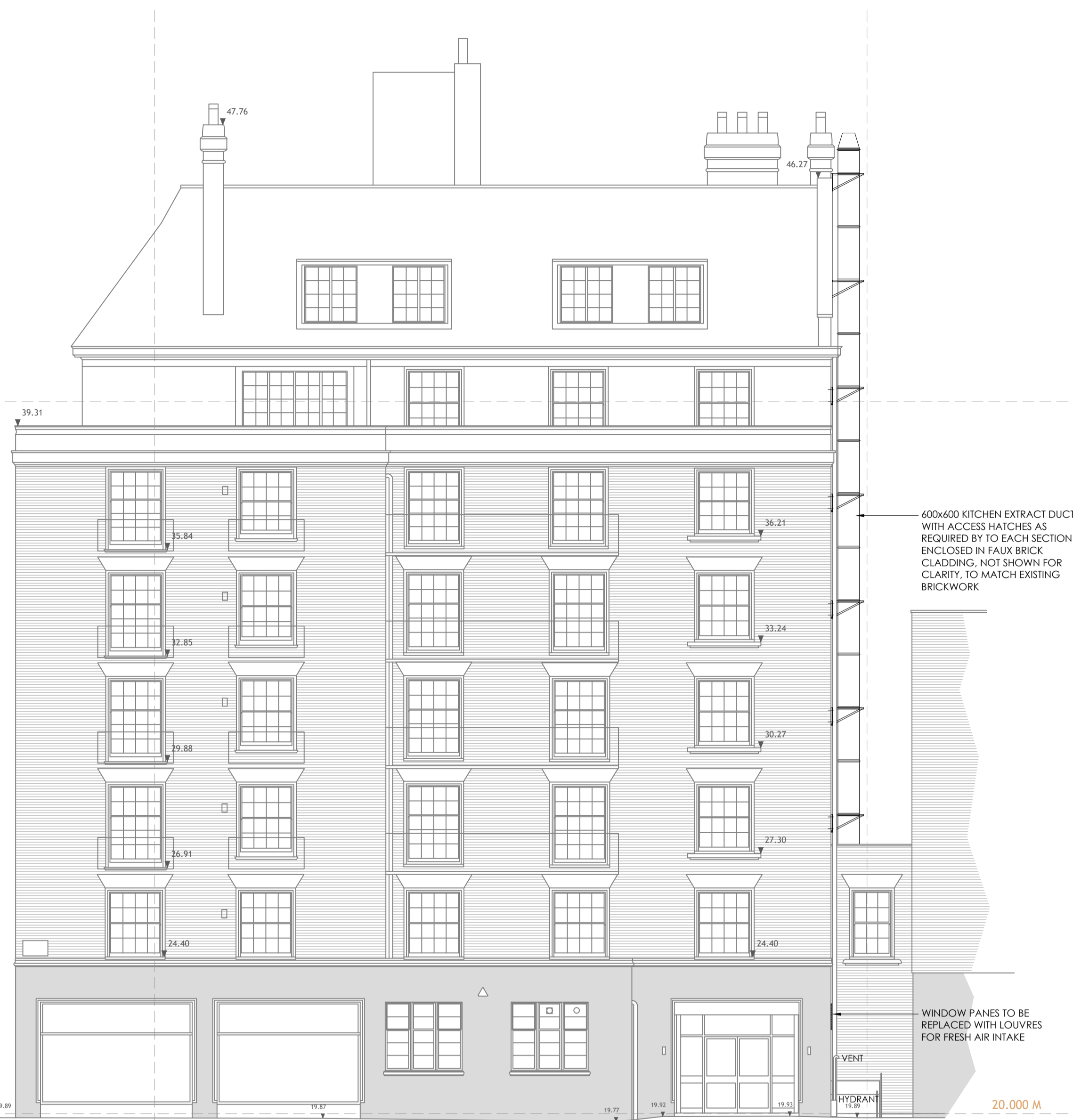
ELEVATION 2 - ALONG REEVES MEWS SCALE 1:100 @ A1
