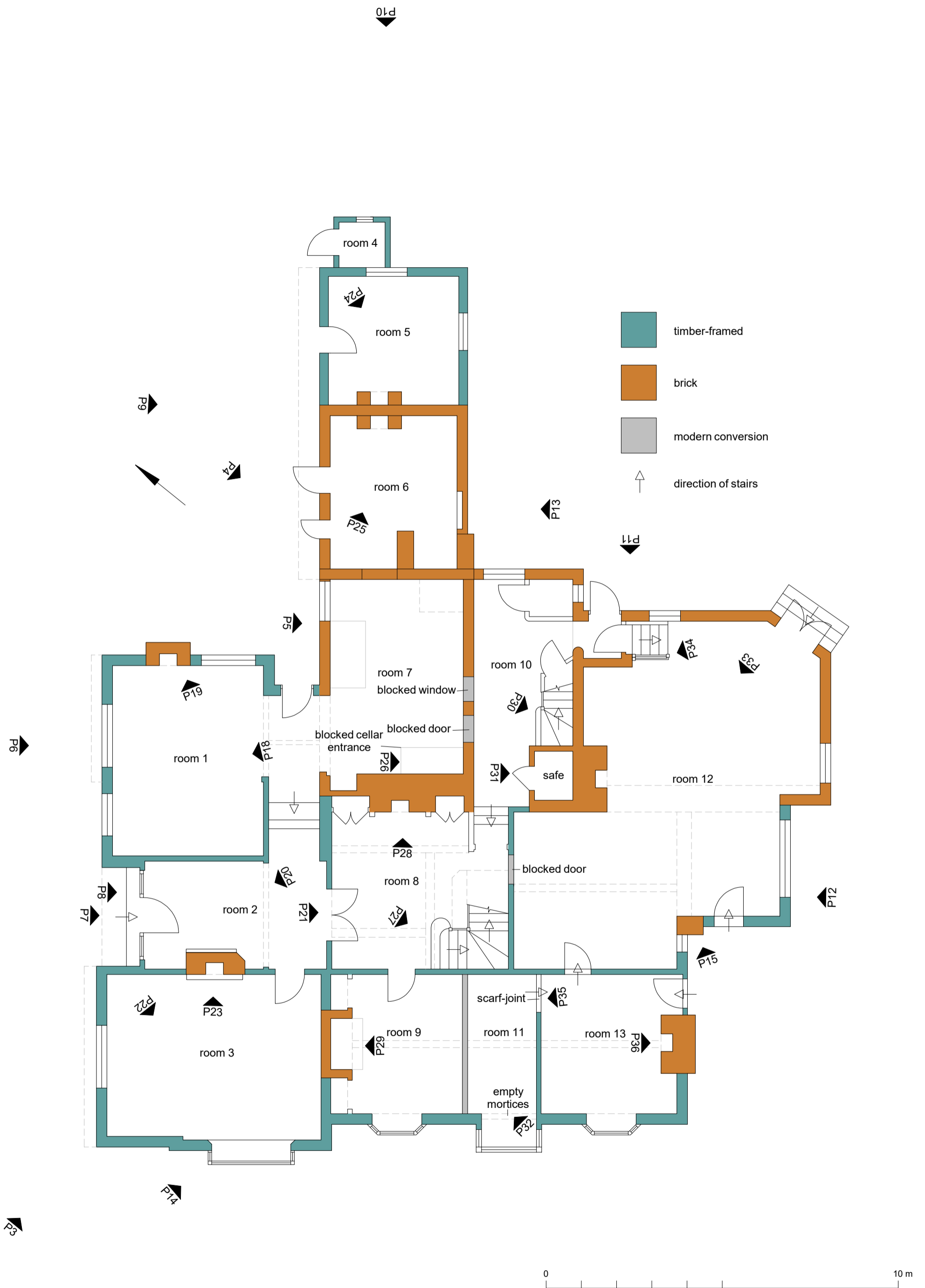
Fig 3 Ground floor plan. Location and direction of photographs reproduced in the text shown.
