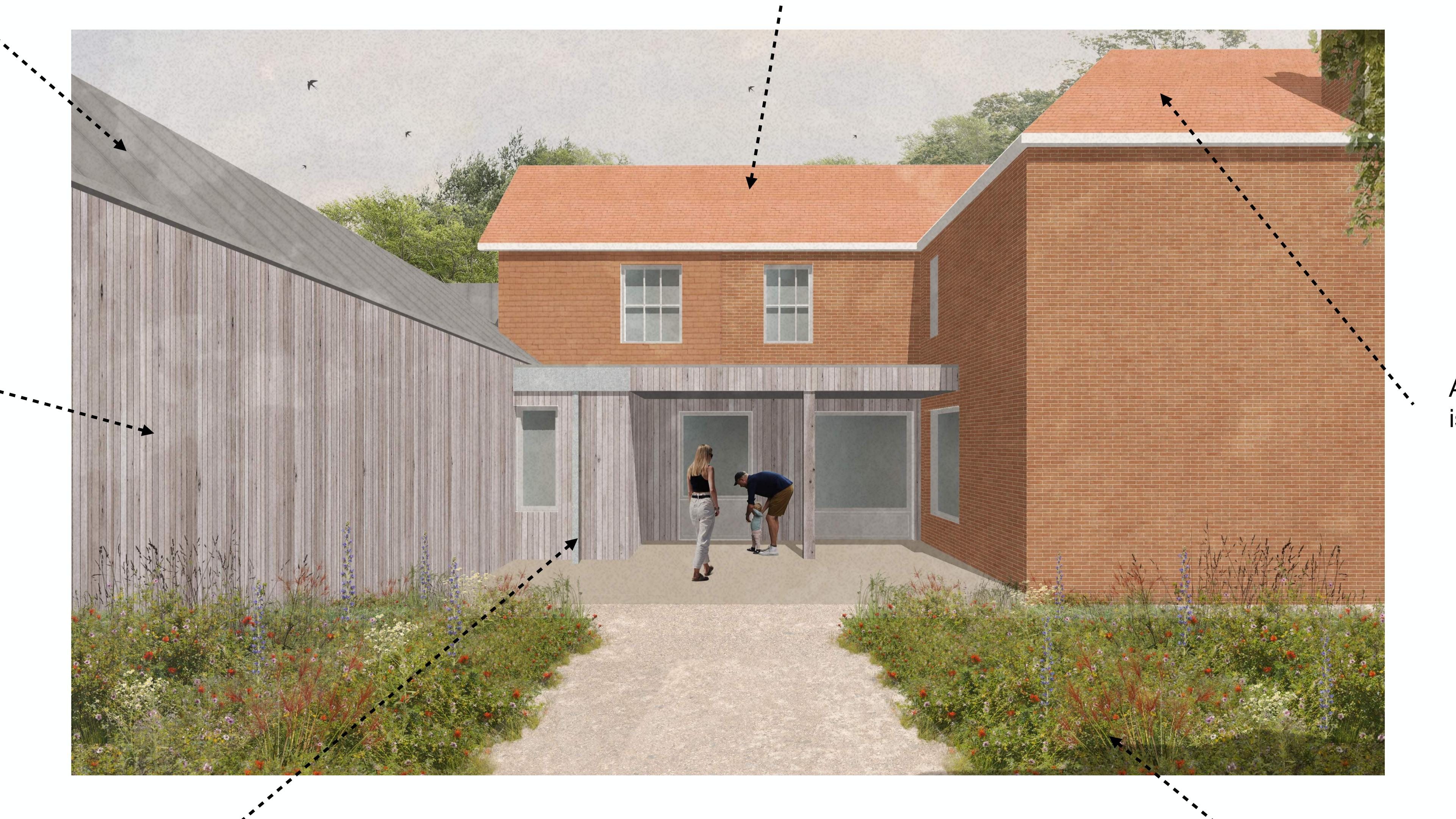
A new Pantile roof to match existing is proposed.
