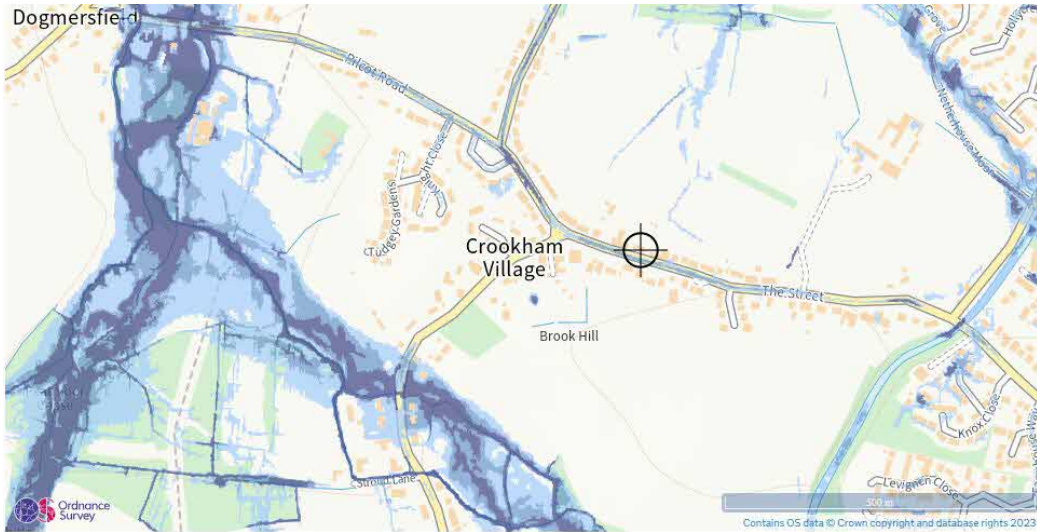
Extent of flooding from surface water
