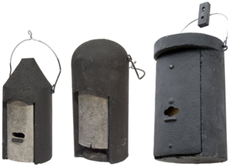
Figure 1. Left to right, the 2F, 2FN and the 1FS bat boxes produced by Schwegler. These and other brands are available at many on-line wildlife stores. These are constructed of 'woodcrete' (a mixture of cement and woodchip) and are designed to be durable and replicate the stable thermal properties of trees and buildings. They may be attached to trees or buildings.
