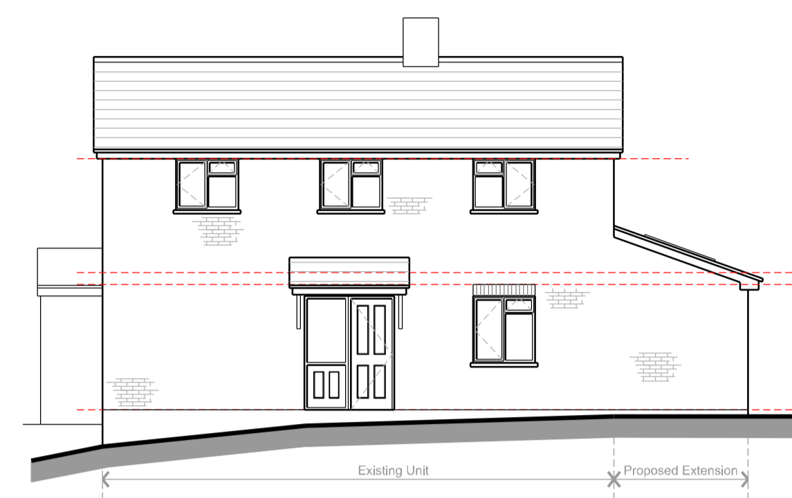
Proposed South Elevation (1:100)
