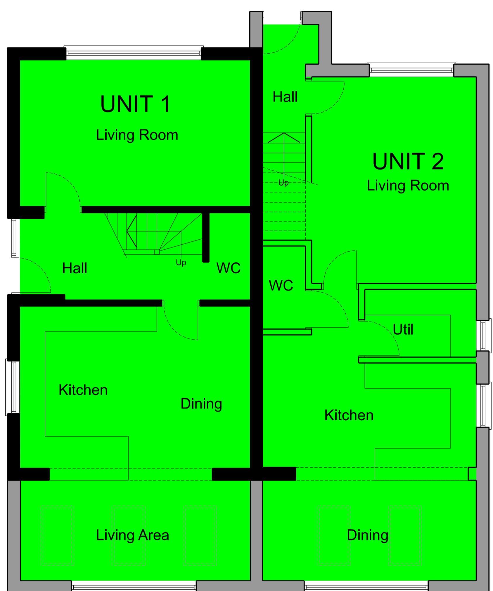
Proposed Ground Floor Plan (1:50)
