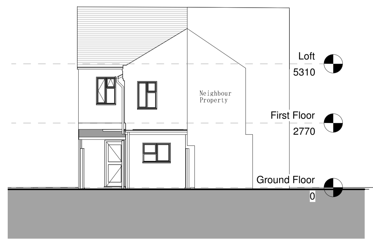
8 Existing - West Elevation 1 : 100
