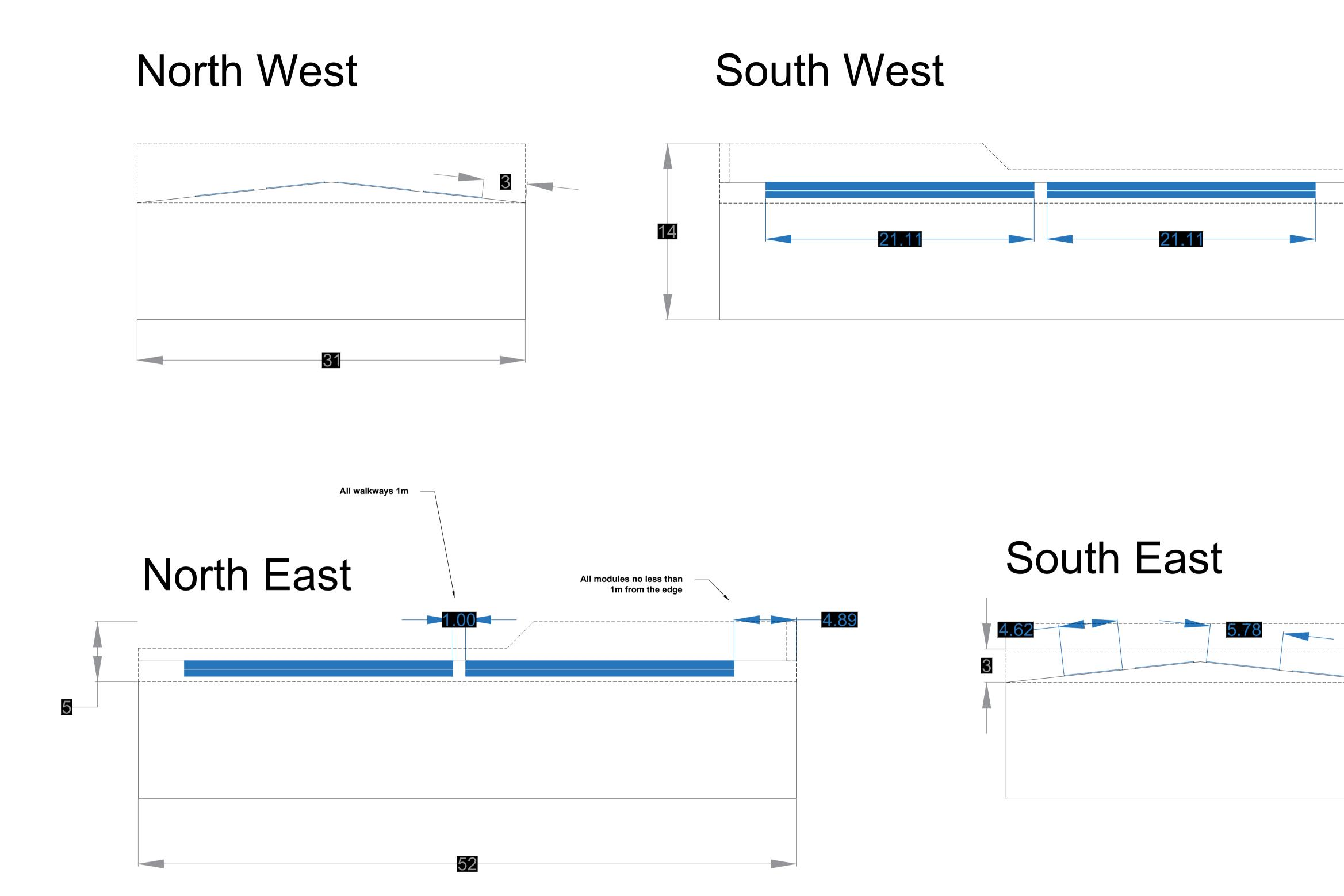
**Roof Pitch:** 10° Eaves Height: 9 Meters Roof Type: Steel Trapazoidal Inverter Location: North West & North East Permanent Roof Access: Unknown
