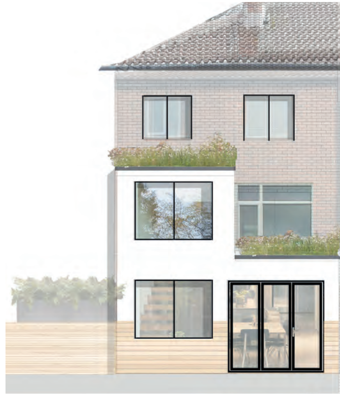
External view of the proposed rear elevation showing the contrasting render and timber cladding to the building
