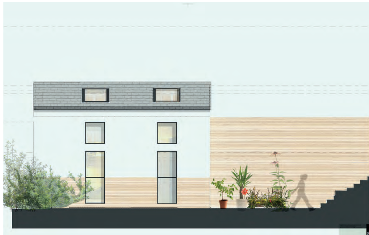
External side view of the garage showing new render and timber cladding to allow for
