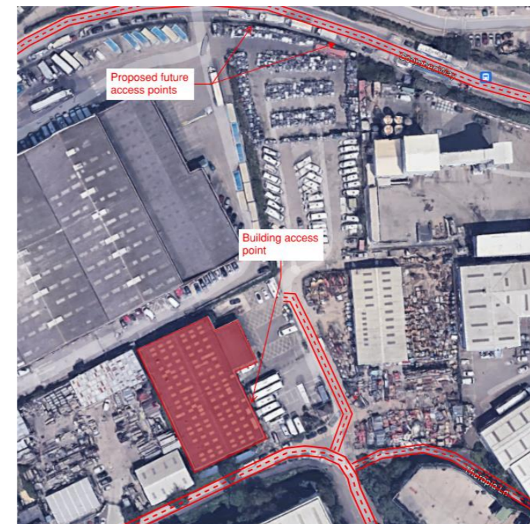
Figure 3 - Indicative fire vehicle access route
