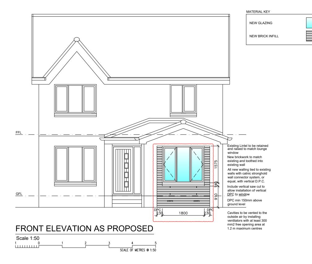
Note: The contractor will be held to have examined the site and determined all dimensions and levels before commencing construction work. No assumption should be made without reference to the architect. No dimensions should be scaled from drawing.
