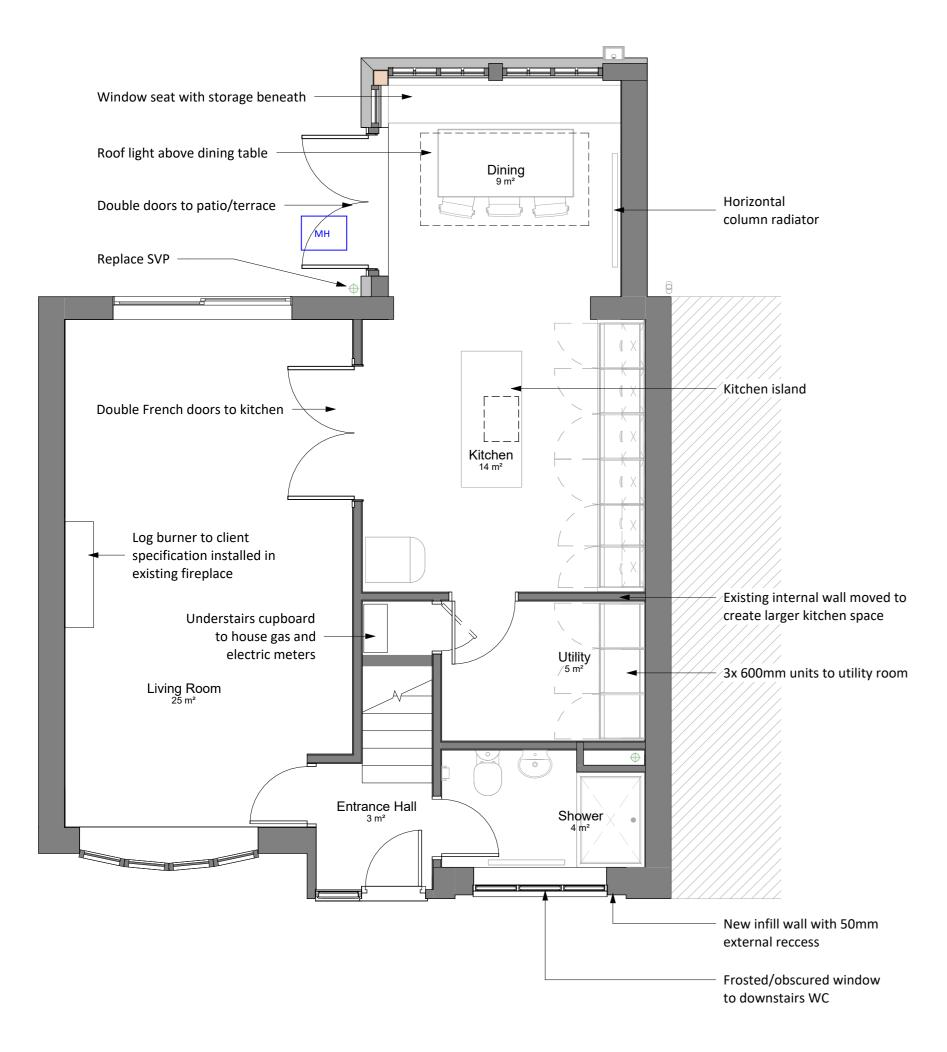
00-Proposed Ground Floor Plan 1:50 01-Proposed First Floor Plan 1:50 Responsibility is not accepted for errors made by others in scaling from this drawing. All construction information should be taken from figured dimensions only.
