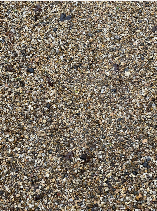
05 The Existing gravel: The resurfaced paths will have a porous asphalt with 'rolled in' aggregate of a size, colour and texture similar to the existing paths
