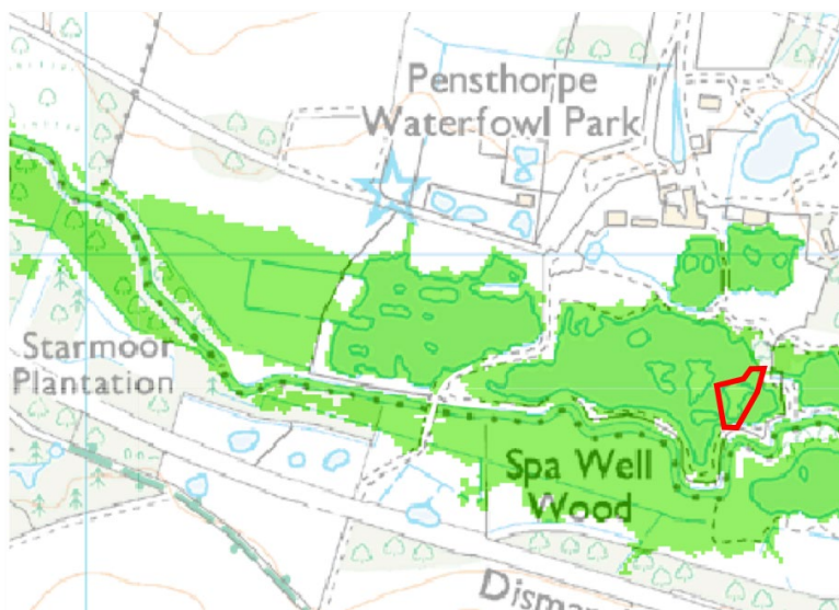
Figure 4: Annotated extract from NNDc SFRA Flood Map – sheet NN30. Area shaded green denotes extent of Flood Zone 3b (functional floodplain)
