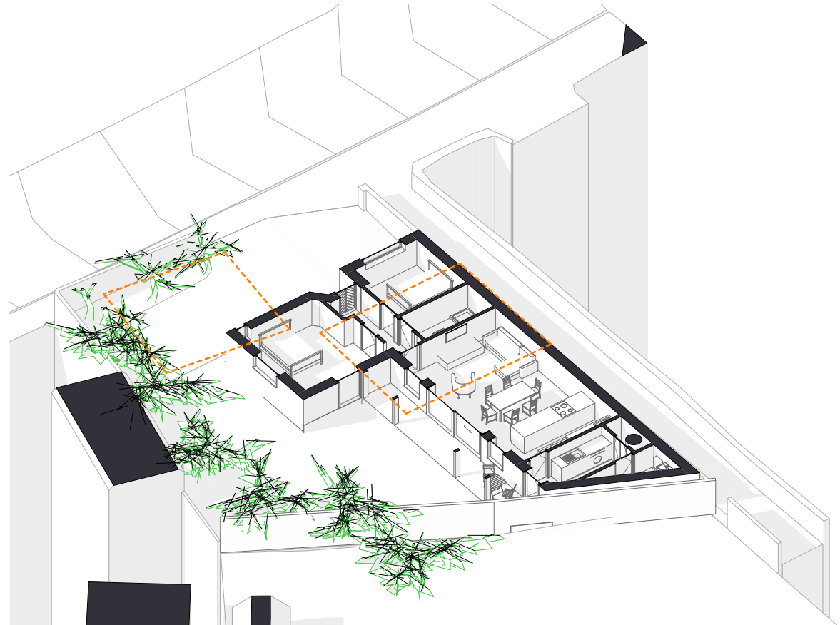
axonometric of proposed layout_ground floor orange dashed lines indicate outline of existing development
