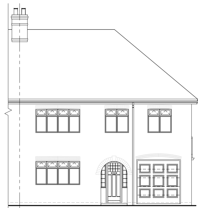
Existing Northeast (front) Elevation 1:100
