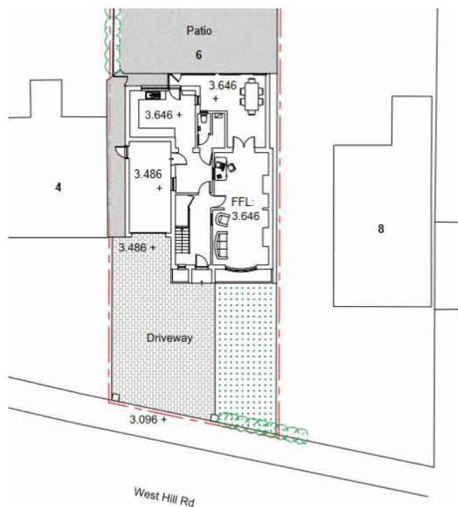
Proposed finished floor levels
