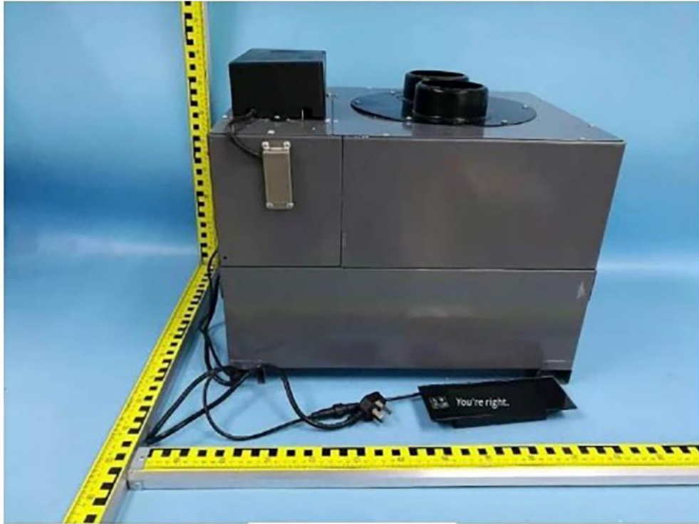
Main inspection model JK-185 appearance (This product is installed inside the oil fume cleaning table, the test finger can only touch the smoke pipe of this appliance during normal use)
