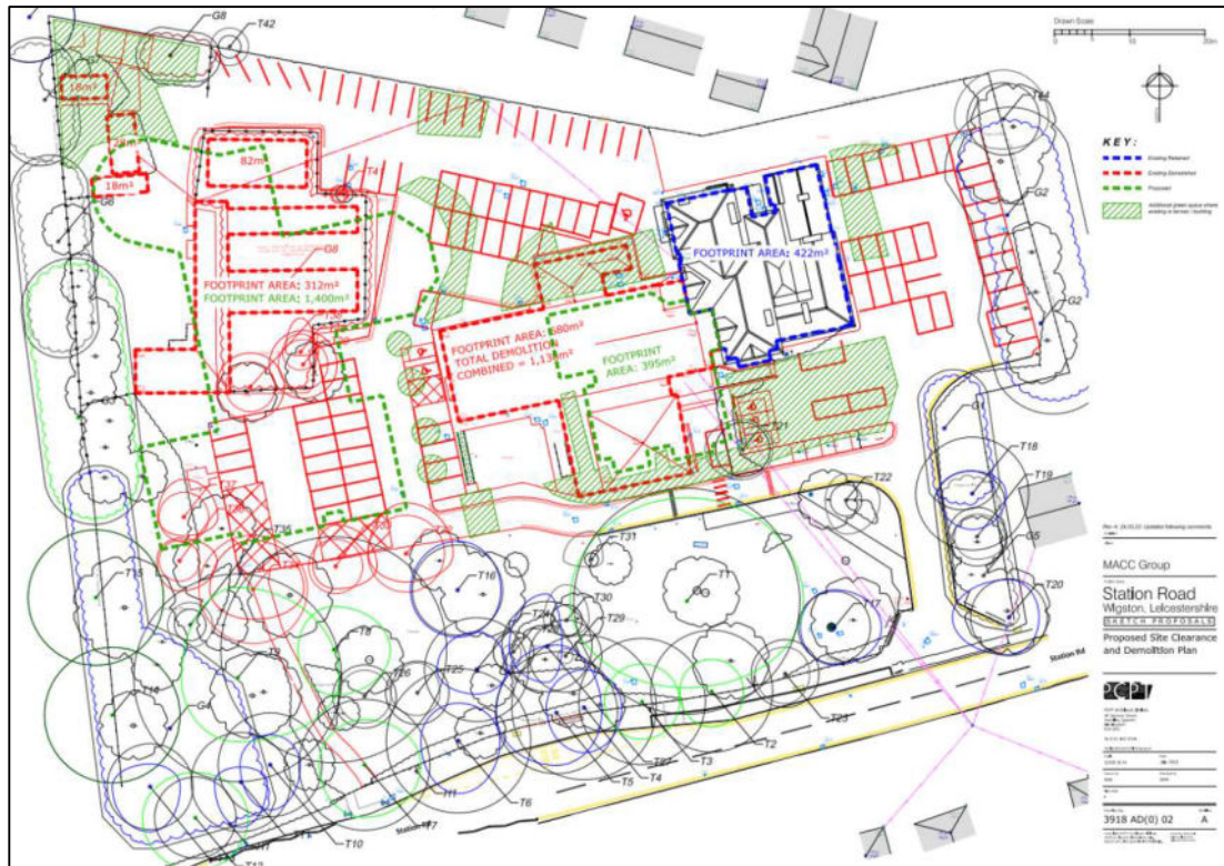
Figure 1-4: Proposed Site Clearance and Demolition Plan
