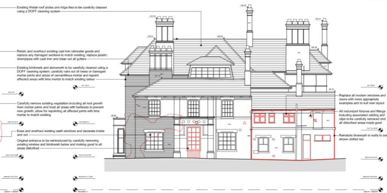
EXISTING EAST ELEVATION 1:100
