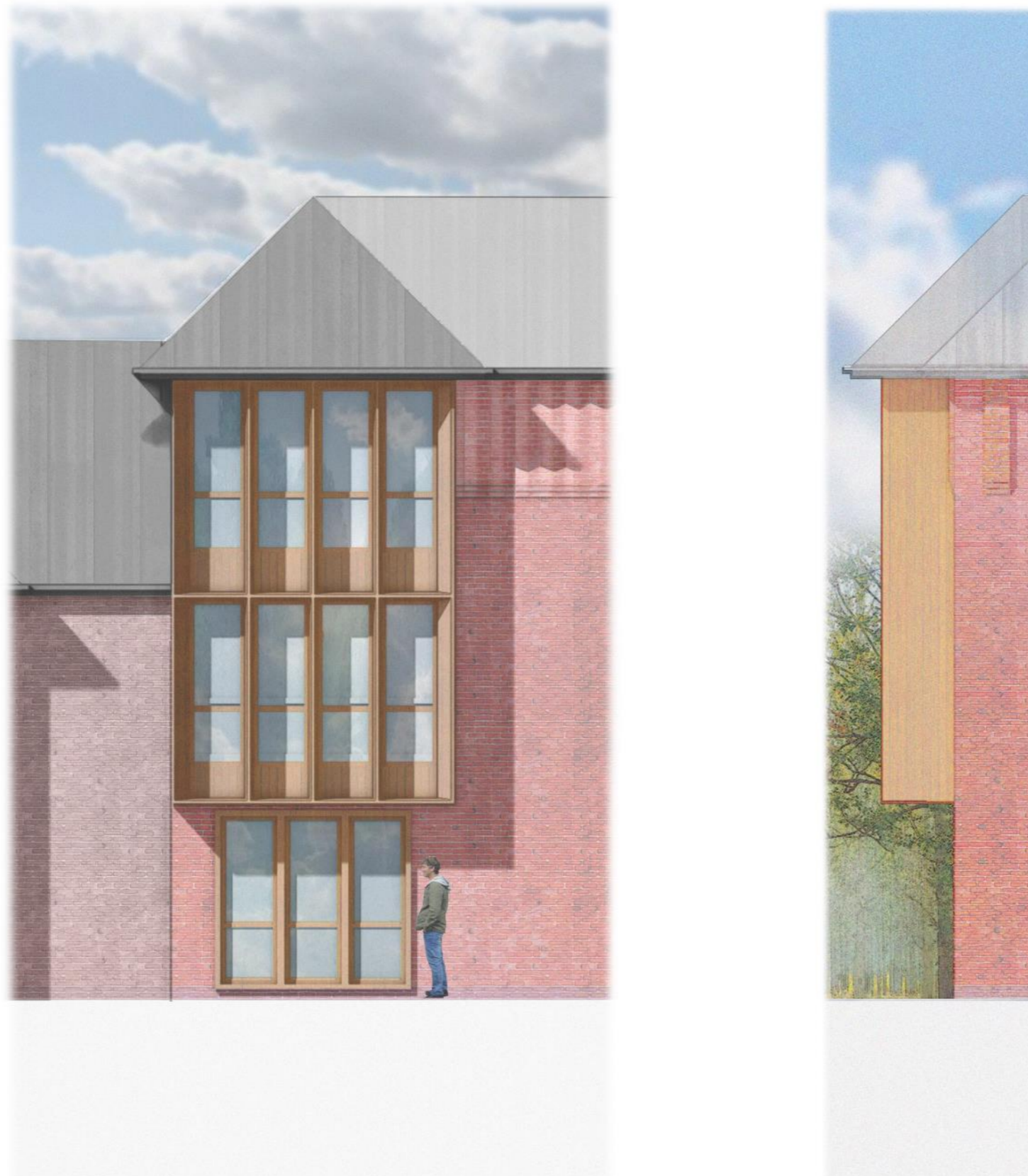
Figure 26: Illustrations of a typical bay window to the new extension to Bushloe House.
