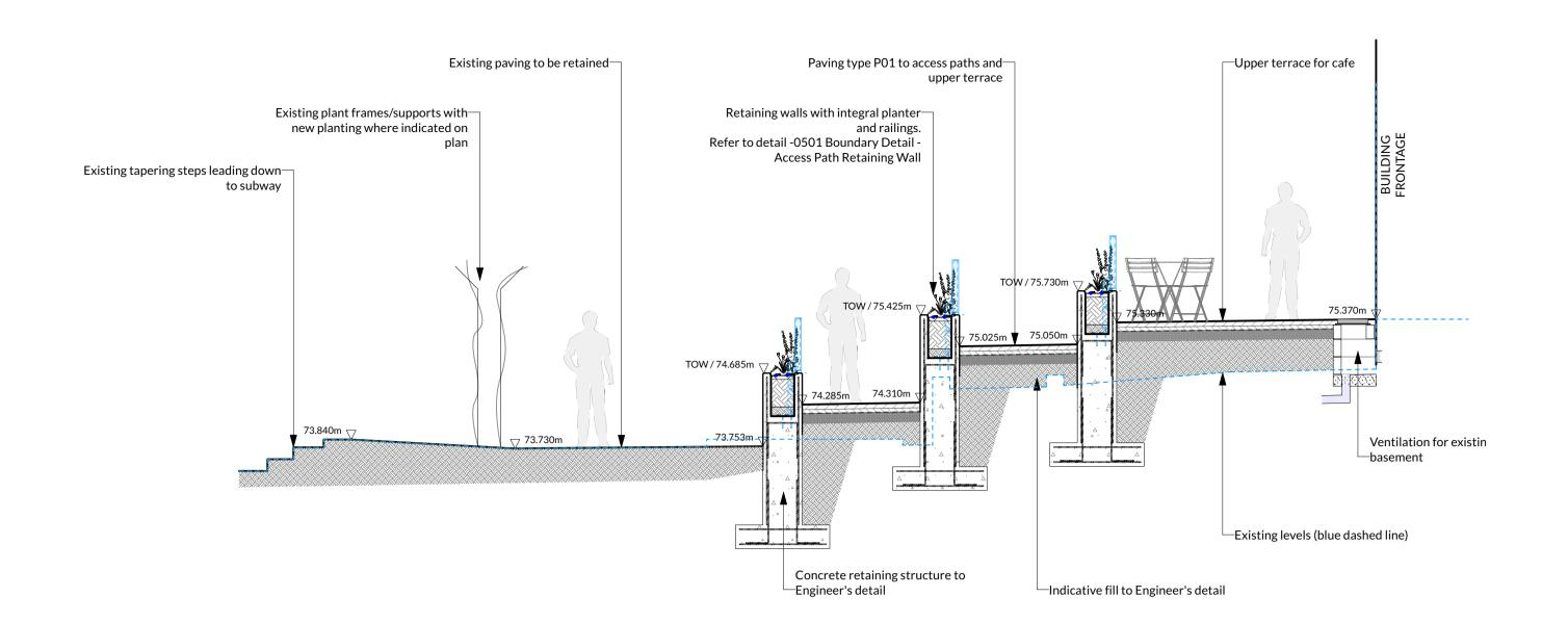
Section Through Access Path and Retaining Walls Scale 1:50 @ A1
