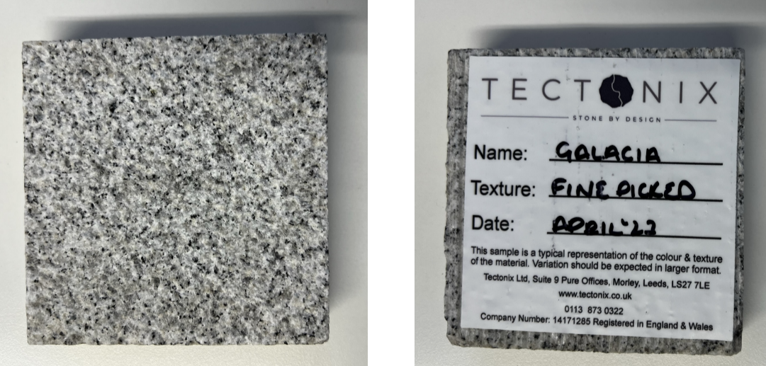
Precedent Image of Granite 'Galacia' Tactile Paving To Corduroy Tactile Paving Scale: NTS at A1
