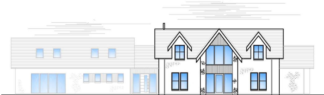
Symmetrical Ground Floor Windows with mullions
