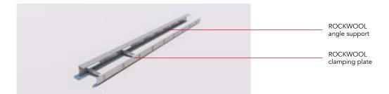
For fixing to timber, the ROCKWOOL clamping plate is used, compressing the barrier to the timber, fixed at 450mm centres using No. 10 woodscrews.
