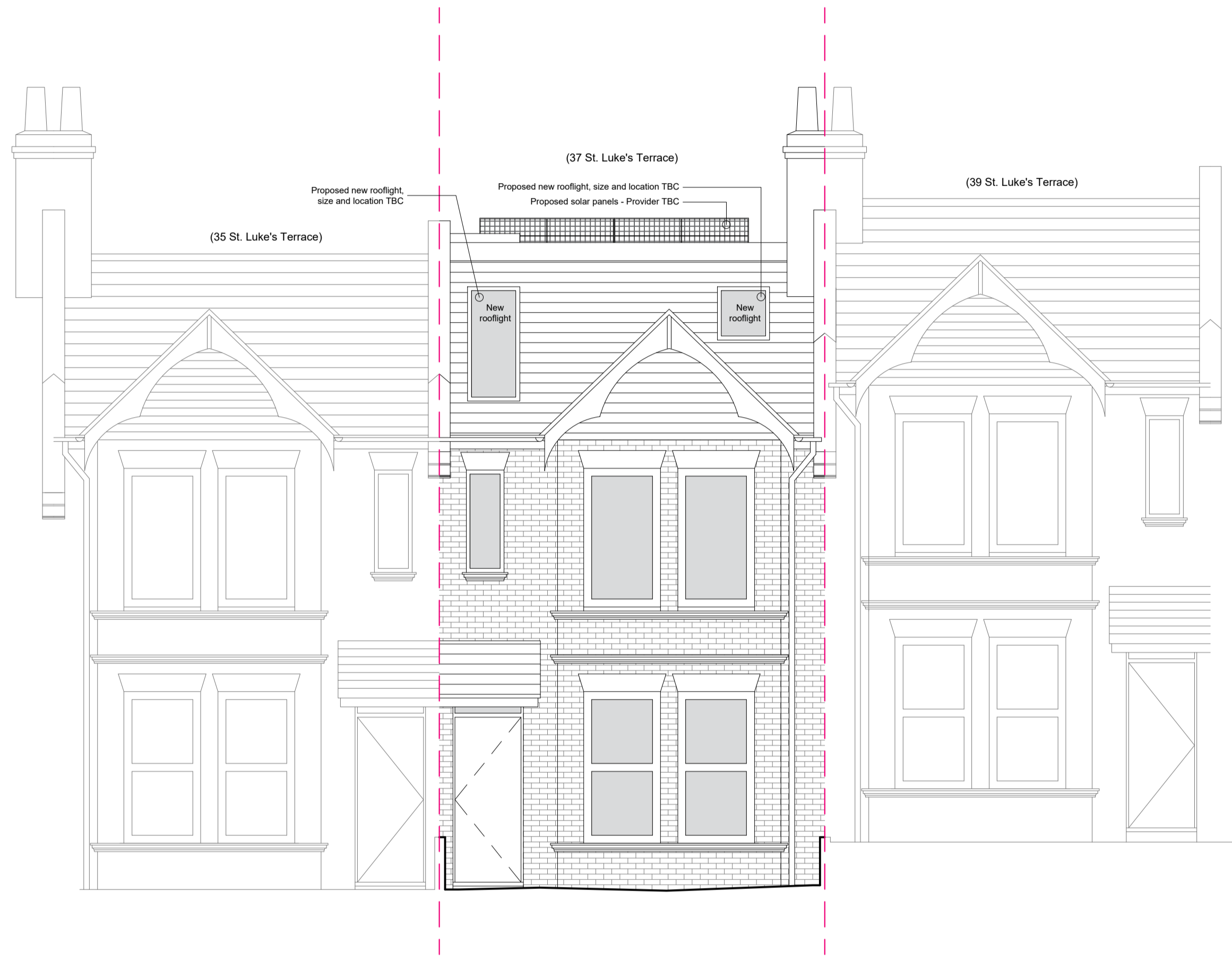
PROPOSED FRONT ELEVATION (SW) 1:50 @ A1
