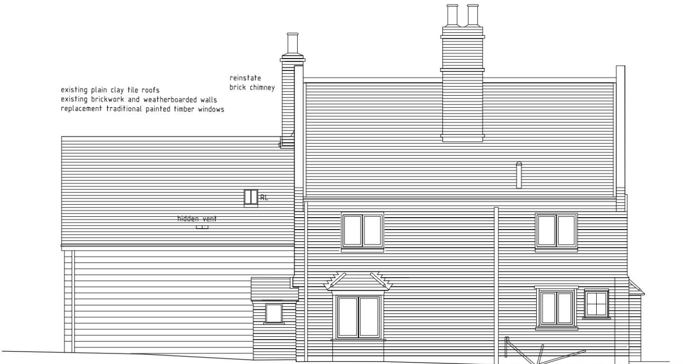
WEST ELEVATION (REAR)
