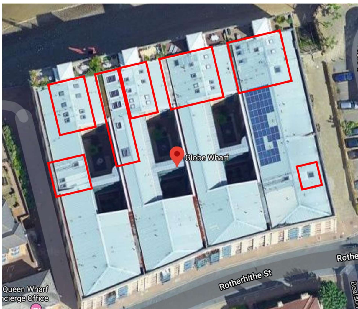
Image 3 above shows a plan view of the Globe Wharf roof. Roof areas highlighted in red show where roof light windows are currently installed.
